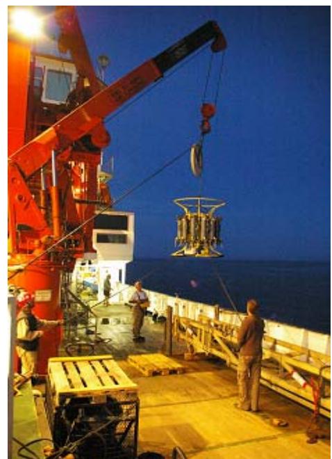
Deployment of the pump CTD. The cable is combined with a 300 m long hose through which the water is pumped on board.
